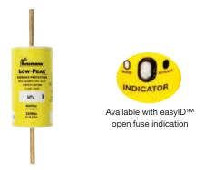
**Description:** Ultimate protection Class J dual element, current-limiting, time-delay fuses available with optional open fuse indication. Time-delay – 10 seconds (minimum) at 500% of rated current.
